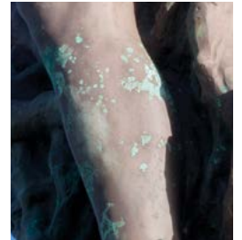
The bright green pustules shown in the detail from this statue suggest active corrosion.
