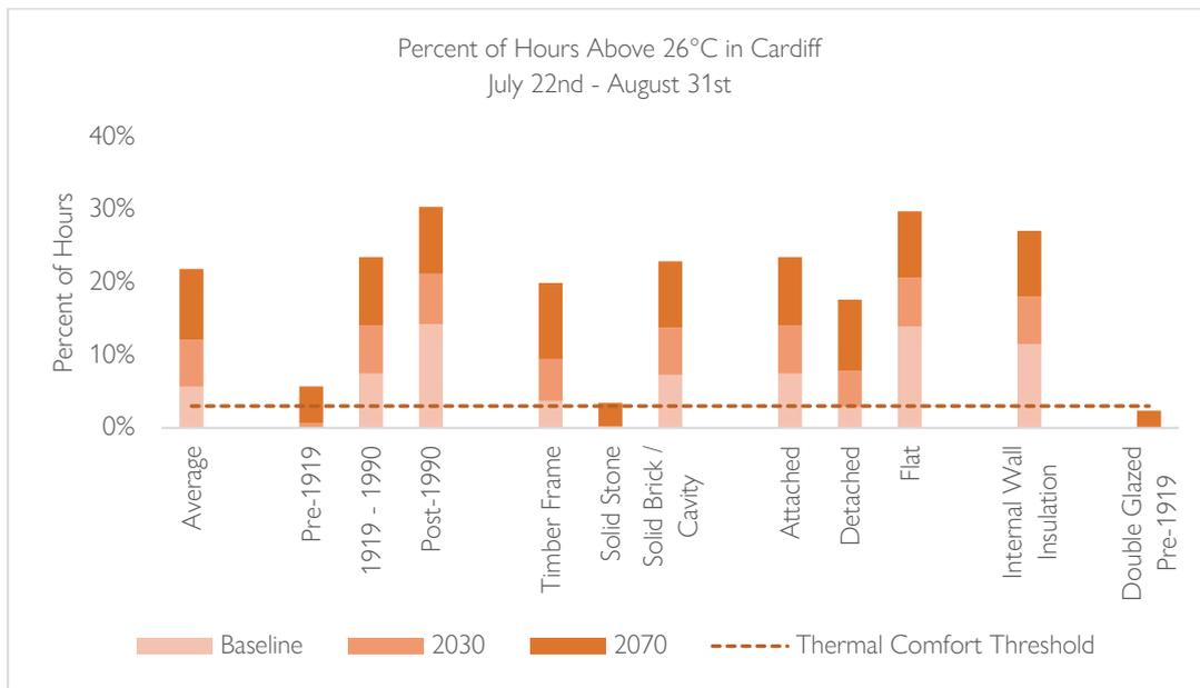
Percent of hours in the study period over 26°C threshold for thermal comfort. Values shown for the average building and eleven building classes. 3% of occupied hours threshold shown for reference.
