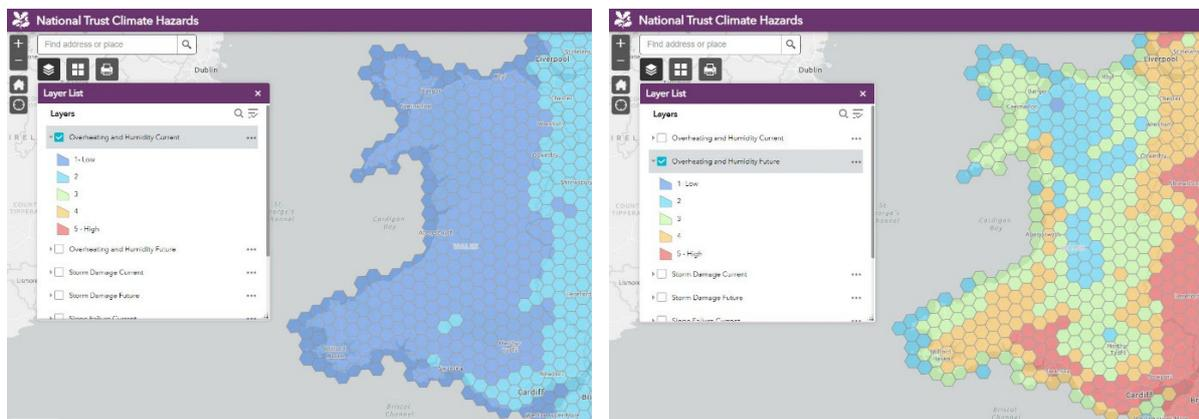
The National Trust Climate Hazards Map. This example shows the likelihood of an overheating and humidity hazard event, now (2020 - left) versus 2060 (right). The event is distributed across 5km hexagonal grids which are ranked from 1-5 (1 = low hazard likelihood, 5 = high hazard likelihood). An overheating and humidity hazard event occurs when daily maximum temperatures exceed 30 degrees Celsius, or average internal humidity falls outside of the 40-60% range, as observed by the Met Office.
