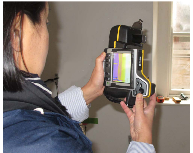
Figure 9: When used in conjunction with air pressurisation testing, thermal imaging can also show clearly where air is leaking through the building envelope.
